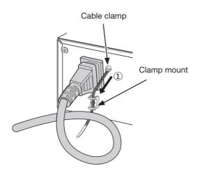
1. Pass the cable clamp (provided) through the clamp mount.
