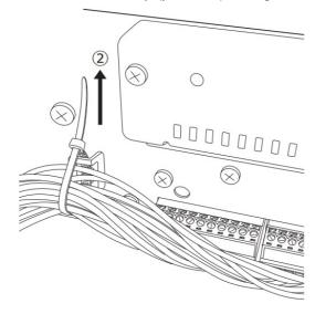
2. Tie the cables of the ALARM/CONTROL terminals and fix with the cable clamp.
