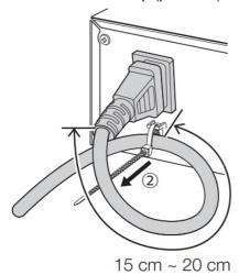
2. Tighten the power cord at 15 cm to 20 cm from the connector and fix it to the clamp mount. Cut the surplus part of the cable clamp as necessary.
