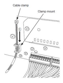
1. Pass the cable clamp (provided) through the clamp mount.
