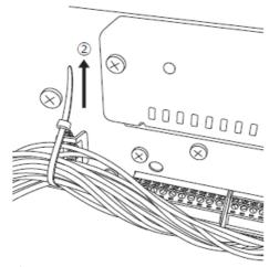
Tie the cables of the ALARM/CONTROL terminals and fix with the cable clamp.
