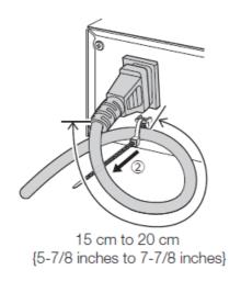
• Fix a 15 cm ~ 20 cm {5-7/8 inches ~ 7-7/8 inches} space from the power cord connector with the attached cable clamp passed through the clamp mount.
