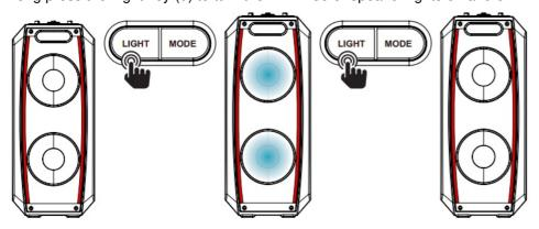
Short press the Light key (9) to change the lighting mode or to switch the LED strip lights on and off. The lighting mode options are slow and fast flashing.
