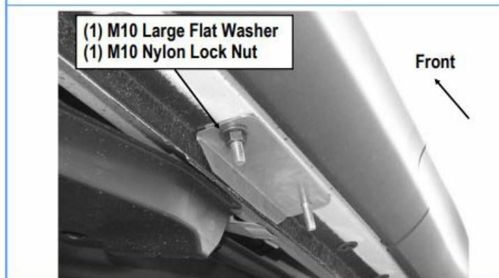
(Fig 9) Locking Plate (DCS1) Installation (Driver Center Side )
