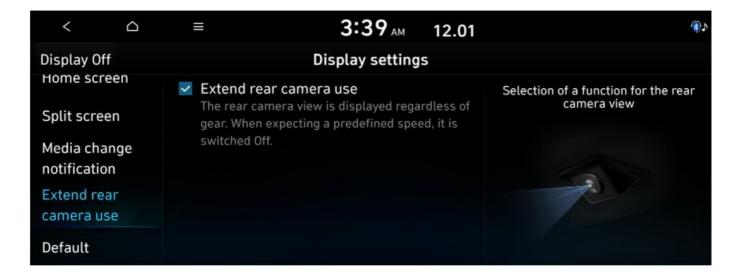
**Note**: When you shift to "P" (Park) or drive at a predetermined speed or faster, the rearview display disappears to display the previous screen.
