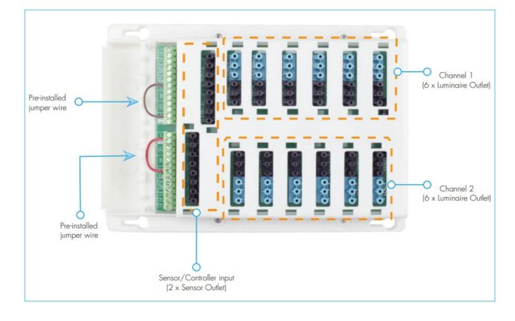
Factory default for SCB03 comes with 2 pre-installed jumper wires. The brown wire short-connects Switched L1 and L1 together, the red jumper wire short-connects Switched L2 and L2 together. With these jumper wires, user can freely choose different dimming control method and also freely switch between DALI control and 0/1-10V control.
