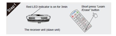
• Short press the "Learn/Erase" button on RC to activate pairing mode, and the receiver unit will flash once every
