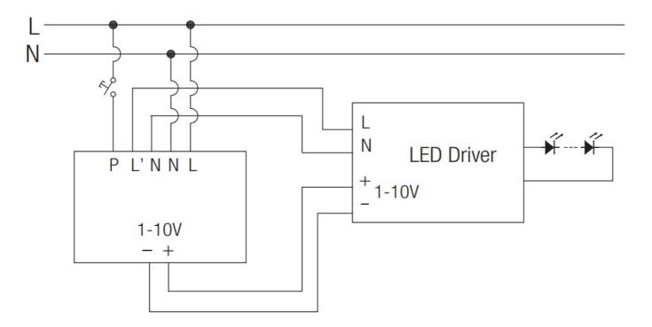
**Note:** if neither function 4.3 nor 4.4 is desired, simply leave the "push" terminal disconnected.
