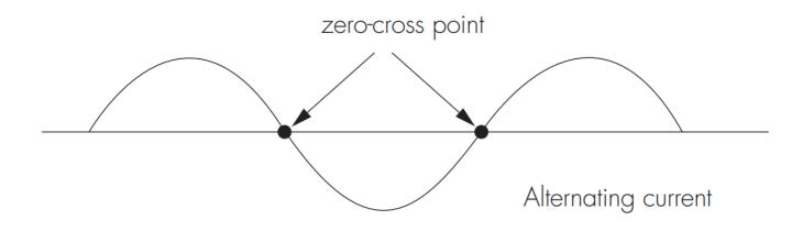
Designed in the software, sensor switches on/off the load right at the zero-cross point, to ensure that the in-rush current is minimised, enabling the maximum lifetime of the relay
