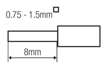
To make or release the wire from the terminal, use a screwdriver to push down the button.
