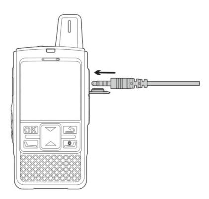
NOTE: To ensure optimum waterproof and dustproof performance, close the audio jack cover after disconnecting the audio accessory.
