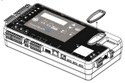
Figure 14. Remove OXI Receiver Cover
