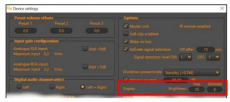
OLED displays are very sensitive to burn-in symptoms, such as permanent discolouring, if white or brightly coloured logos are used at high brightness levels. To avoid burn-in symptoms, we recommend that you set the level to 6 or lower.
