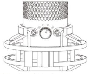
Rotate the polar pattern knob to select one of the four polar patterns.
