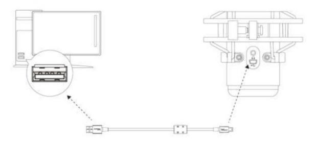
Connect the microphone to a USB port on the PC or Mac with the included USB cable.
