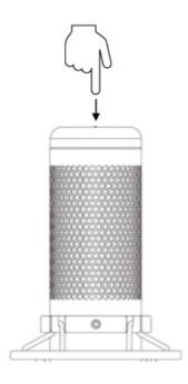
Tap the top of the microphone to mute/unmute the microphone. The microphone LED will indicate the current mute status of the microphone.
