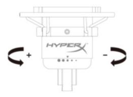
Rotate the gain control knob to adjust the gain of the microphone.
