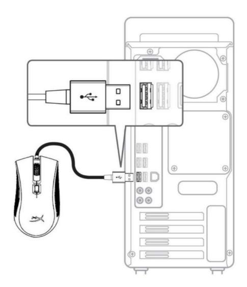
1. Connect the USB connector to the computer.
