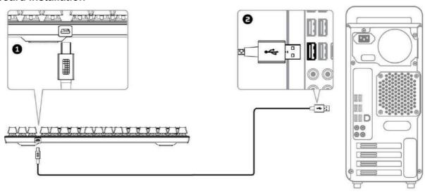
1- Connect the Mini USB connector to the keyboard.
