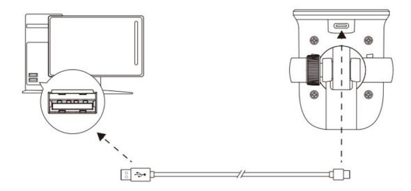
Connect the microphone to a USB port on the PC or Mac with the included USB cable.
