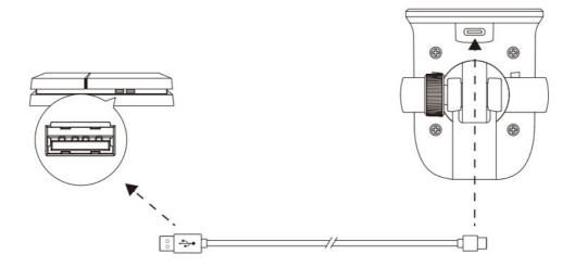
Connect the microphone to a USB port on the PS4 $^{\text{TM}}$  with the included USB cable. To ensure the microphone is configured correctly on the PS4 $^{\text{TM}}$ , follow the steps below:
