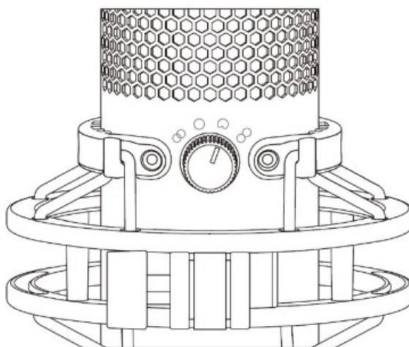
Rotate the polar pattern knob to select one of the four polar patterns.
