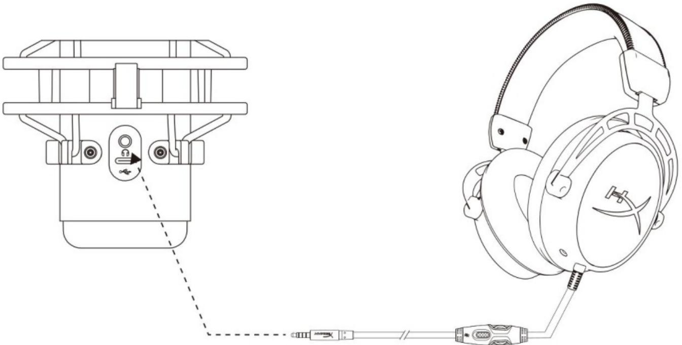
Connect headphones to the headphone jack on the microphone for microphone monitoring and playback audio.
