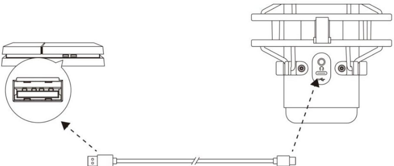
Connect the microphone to a USB port on the PC or Mac with the included USB cable.
