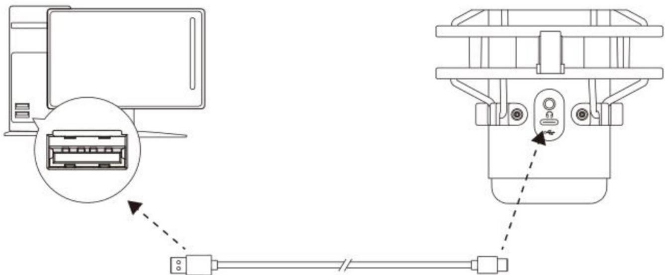
Connect the microphone to a USB port on the PS4 with the included USB cable. To ensure the microphone is configured with the most optimal settings on the PS4, follow the steps below:
