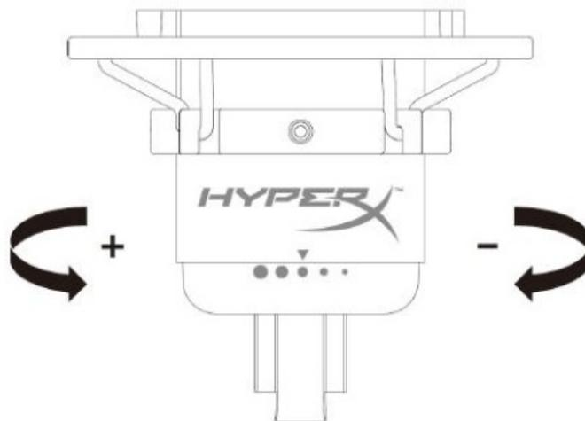
Rotate the gain control knob to adjust the gain of the microphone.
