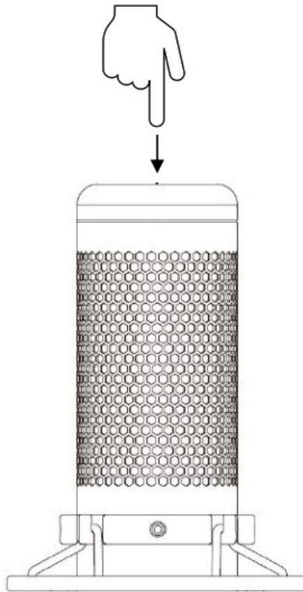
Tap the top of the microphone to mute/unmute the microphone. The microphone LED will indicate the current mute status of the microphone.
