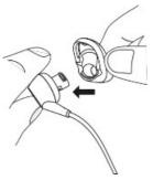
3. Pull the stabilizer flap to stretch the nozzle over the hook
