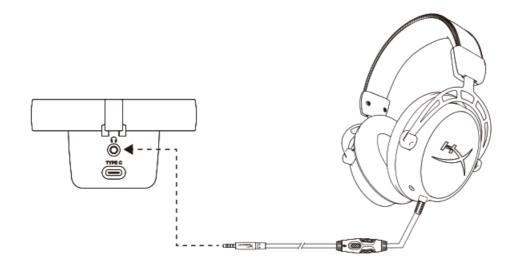
Connect headphones to the headphone jack on the microphone for microphone monitoring and playback audio. **Selecting a Microphone Polar Pattern**
