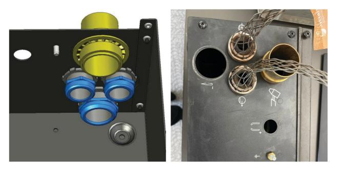
**Step 7**Remove the nuts using a 7/16 inch socket and pull to remove the wires. Discard the nuts and wires into the mixed metal recycling waste stream.
