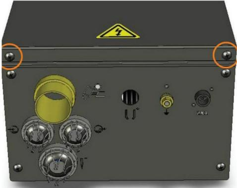
**Step 4**Remove the bolts and nuts using the T20 TORX driver bit and a 5/16 inch socket. Discard the bolts and nuts into the mixed metal recycling stream.
