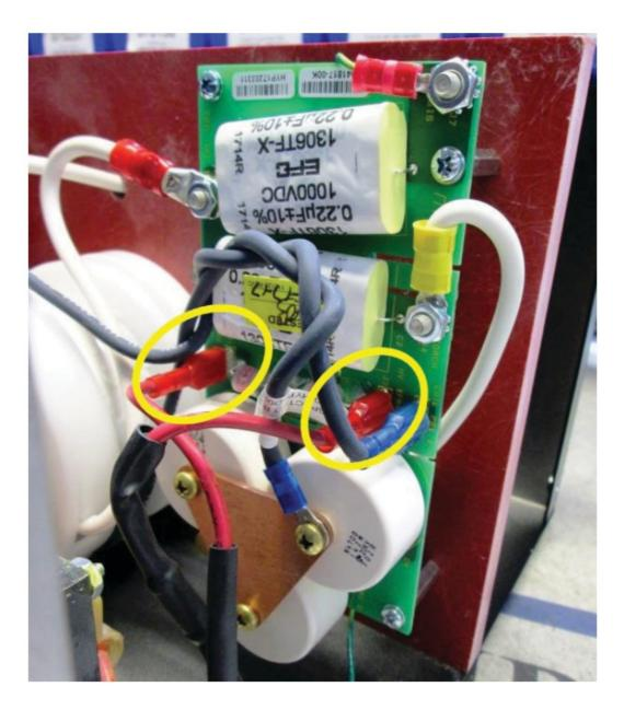
**Step 6 Note:** There is no need to remove the wires. You can optionally recycle them into the mixed metal recycling stream.
