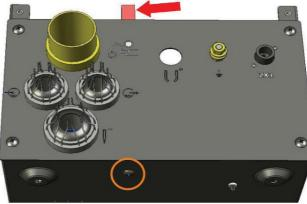
**Step 5**Remove the nuts and screws using a 11/32 inch socket and a Phillips screwdriver. Pull to remove the wires. Discard the nuts, screws, and wires into the mixed metal recycling stream. Discard the PCB into the E–waste recycling stream.
