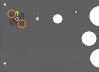
**Step 9**Remove the screws and nuts using a Phillips screwdriver and a 11/32 inch socket. Discard the screws and nuts into the mixed metal recycling stream.
