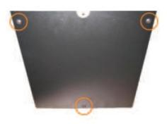
**Step 4**Remove the bolts and nuts using the T20 TORX driver and a 5/16 inch socket.
