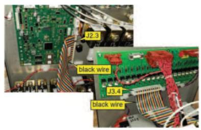
**Step 7**Remove the nuts using a 7/16 inch socket and pull to remove the wires.
