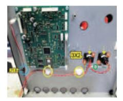
**Step 11** Remove the nuts using a 1/4 inch socket and a 7/16 inch socket.
