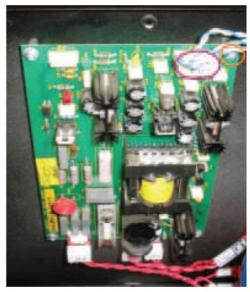
**Step 5**Remove the nuts and screws using a 11/32 inch socket and a Phillips screwdriver. Pull to remove the wires.
