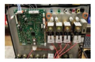
**Step 10**Remove the screws and nuts using a Phillips screwdriver and a 1/32 inch socket.
