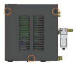
**Step 3** Remove the bolts using the T20 TORX driver.
