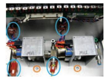
**Step 9**Remove the screws and nuts using a Phillips screwdriver and a 11/32 inch socket.
