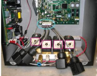
**Step 4**Remove the screws using a Phillips screwdriver and cut all cable ties.
