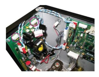
**Step 3**Loosen the screws with a Phillips screwdriver. Pull on the cables to remove them from their connectors.
