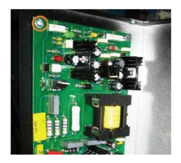
**Step 7**Remove the nuts using the ½ inch, 5/16 inch, and 7/16 inch sockets. Discard the nuts into the mixed metal recycling stream.
