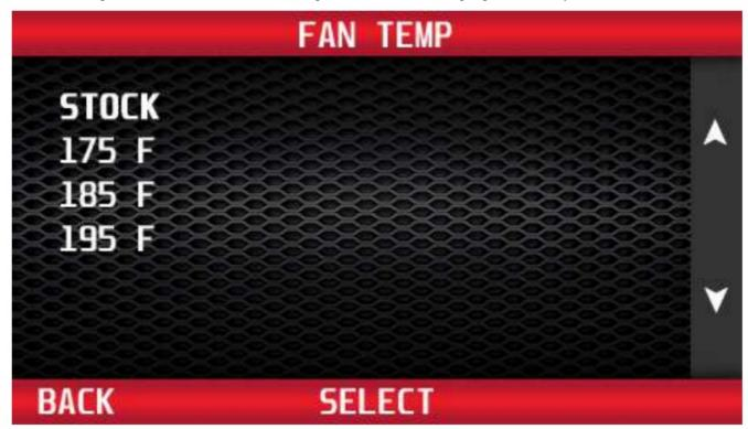
Use the buttons to the right of the screen to select the desired temp thermostat. Press 'Select' to save the chosen thermostat temp.
