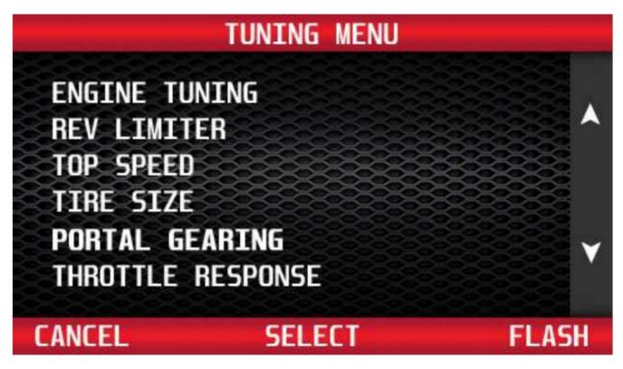
From the Tuning Menu, use the buttons to the right of the screen to highlight Portal Gearing. Press the 'Select' button to recalibrate the speedometer reading for installed portal gears.
