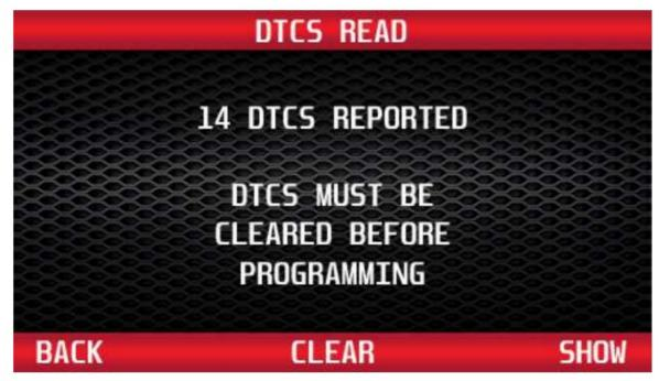
Use the buttons to the right of the screen to scroll up or down and review each DTC. To see a definition of each DTC, press the 'More' button. The programmer will display a description of the DTC. To clear all DTCs, press the 'Clear' button.
