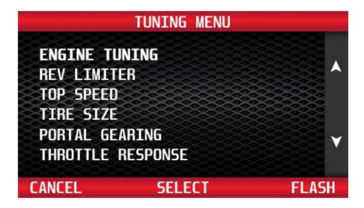
From the Main Menu, use the buttons to the right of the screen to highlight Engine Tuning. Press the 'Select' button to choose an optimized engine tuning program.
