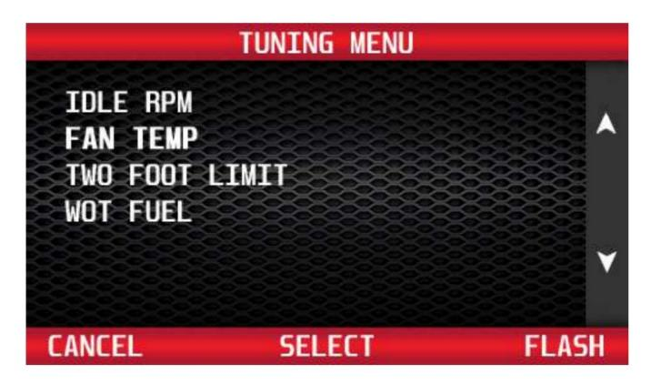
From the Tuning Menu, use the buttons to the right of the screen to highlight Fan Temp. Press 'Select' to choose.
