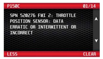
NOTE: Necessary repairs must be made to the corresponding DTC code(s) to properly clear the DTC(s). Make these repairs and clear all DTCs with the programmer BEFORE programming the vehicle.
