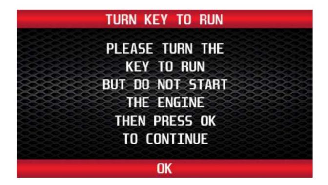
Turn the key to the 'Run' position and select 'OK' using the middle bottom button.
