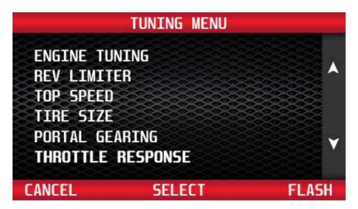
From the Tuning Menu, use the buttons to the right of the screen to highlight Throttle Response. Press 'Select' to choose.
