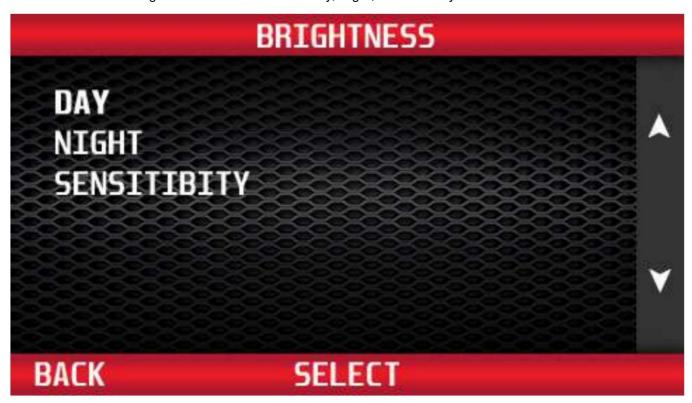
Use the buttons to the right of the screen to adjust the brightness of the display screen, from 1 to 9. Press the 'Back' button to return to the previous menu.
