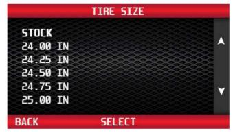
From the Tuning Menu, use the buttons to the right of the screen to highlight Tire Size. Press the 'Select' button to recalibrate the speedometer reading for installed non-stock tire sizes. Use the buttons to the right of the screen to highlight the desired tire size. Press 'Select' to save the chosen value.
