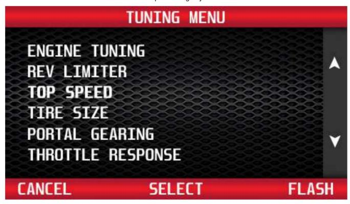
From the Tuning Menu, use the buttons to the right of the screen to highlight Top Speed. Press the 'Select' button to adjust the top speed limiter.
