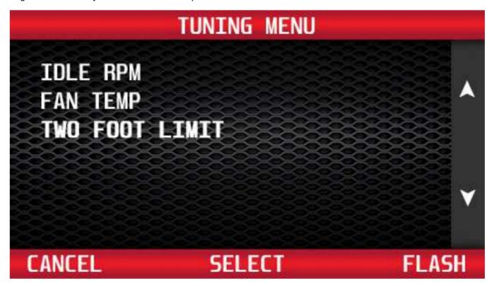
From the Tuning Menu, use the buttons to the right of the screen to highlight Two Foot Limiter. Press 'Select' to choose.
