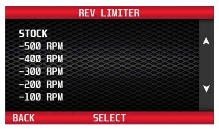
Use the buttons to the right of the screen to scroll up or down and highlight the value to increase or decrease the engine rev limiter. Press 'Select' to save the chosen value.
