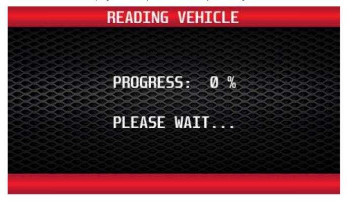
Once the programmer has completed the reading process, it will proceed to the Writing Vehicle mode. Continue to follow the messages on the screen. You may be prompted to turn the key to the 'Run' and 'Off' position during this process.
