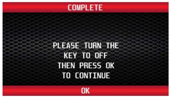
It is now safe to unplug the programmer from the vehicle and start the engine. Make sure the "Check Engine" light on the instrument cluster goes out (If it stays on or flashes, read out the DTCs, and contact Roost Dirt Sports tech support). Warm up the engine and make sure it is running smoothly.
