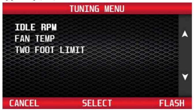
From the Tuning Menu, use the buttons to the right of the screen to highlight Idle RPM. Press 'Select' to choose.
