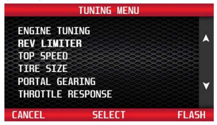
From the Tuning Menu, use the buttons to the right of the screen to highlight Rev Limiter. Press the 'Select' button to adjust the engine rev limiter, in 100 RPM increments.
