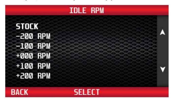
Use the buttons to the right of the screen to select the desired idle RPM. Press 'Select' to save the chosen idle RPM.
