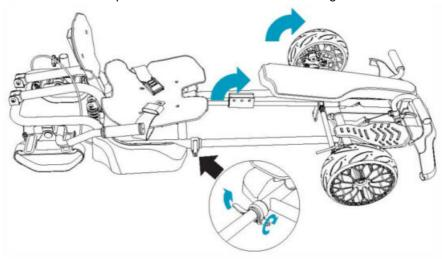
Step 2: Fix the length of the kart and lift the steering wheel to the proper position
