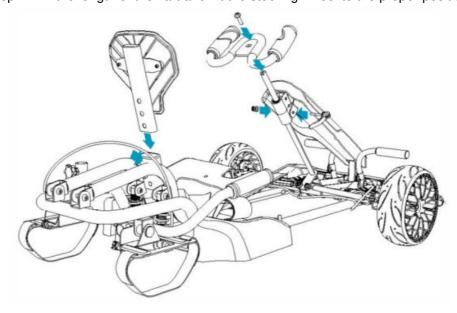
Step 3: After fixing the steering wheel, install the steering wheel and seat successively, the Kart installation completed
