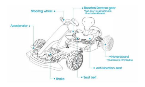
L: 1100-1300mm W: 700mm H: 500mm AdJustable length of the frame.20Dmm
