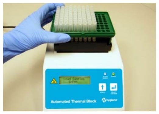
8. The unit beeps once, and the LCD display changes as the thermal block begins equilibrating to 55 °C. While the block is heating, follow the instructions in the BAX System User Guide to add additional lysing reagents to each sample.
