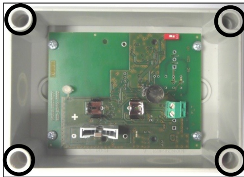
Picture 3 - Wall fixing screw entry points
