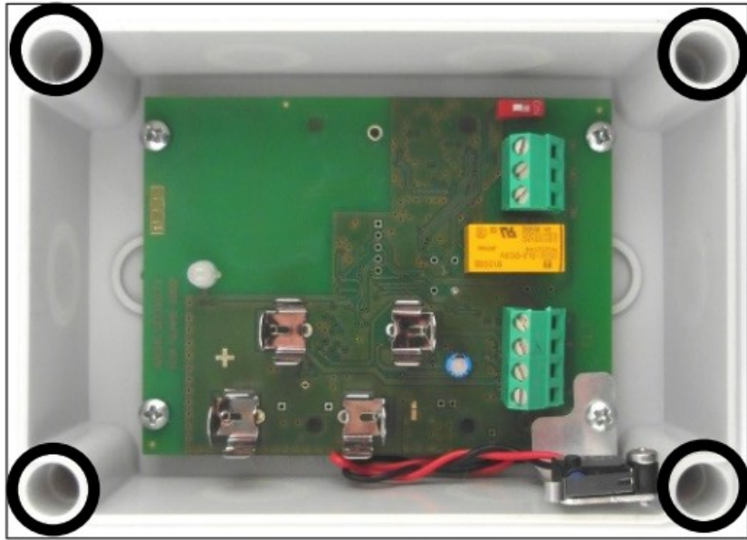
Picture 3 – Wall fixing screw entry points
