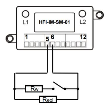
The **HFI-IM-SM-01** single channel supervised input mini-module provides monitoring of normally open contact fire alarm and supervisory devices.
