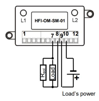
The HFI-OM-SM-01 single channel supervised output mini-module provides control, by closing contacts, of auxiliary devices such as fire shutters.
