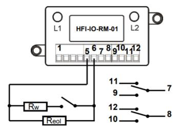
The HFI-IO-RM-01 input and output relay mini-module combine in a single device supervised input and relay output characteristics.
