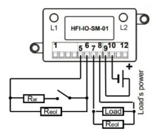
The HFI-IO-SM-01 input and output supervised mini-module combine in a single device supervised input and output characteristics.
