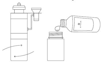
4. Screw and place the bottle back to the diffuser machine.
