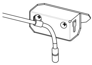
**STEP 2** Secure the sensor on the bracket by pressing it down into the slotted hole as shown above.
