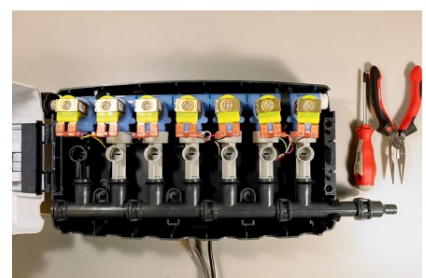
6-product EvoClean - Prepared for maintenance
