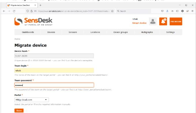
After you click to Save button on the web page, take a pencil or other tool and briefly press the Setup button on the device. It will start blinking (communication with the portal) and finalize device migration process.
