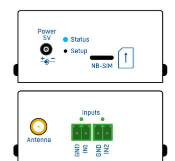
A device for connecting a door or window contact, a PIR motion detector or a smoke or gas detector with a dry contact output. Allows connecting 2 independent detectors. Inputs feature pulse counters for connecting energy meters with an S0 output. **Due to high energy requirements of S0 outputs, external power is required for reliable pulse counting.** Otherwise, reliable operation cannot be guaranteed.
