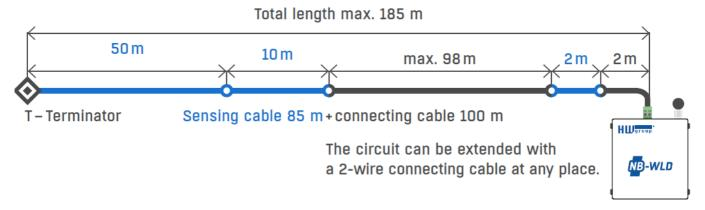
The flood detection is performed every 5 minutes and the estimated battery life are 4 years. If the cable is flooded or disconnected and the device is powered from an external adapter, the red LED lights up. The LED is inactive on battery power.
