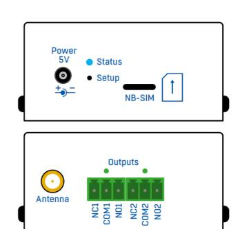
A module with 2 relay outputs controlled from the SensDesk portal over the NB-IoT network. To reduce consumption, the device features two latching relays. For increased reliability, the relays are energized repeatedly every 10 minutes. The device is not suitable for mobile applications. On battery power only, the estimated battery life are 2 years.
