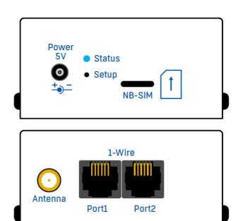
Measurement hub for connecting thermo-meters, humidity sensors or other sensors via the 1-Wire bus. Allows connecting two 1-Wire or 1-Wire UNI sensors (one per port) to measure up to 4 quantities simultaneously.
