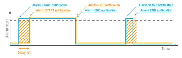
Alarm status notification based on a Delay value:
