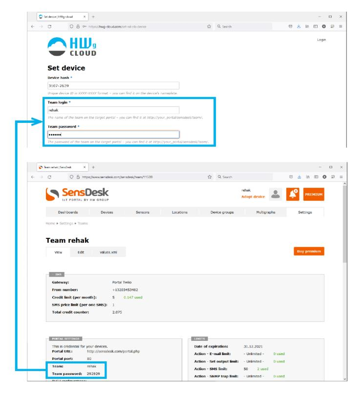
After you click to Save button on the web page, take a pencil or other tool and briefly press the Setup button on the device. It will start blinking (communication with the por-tal) and finalize device migration process.
