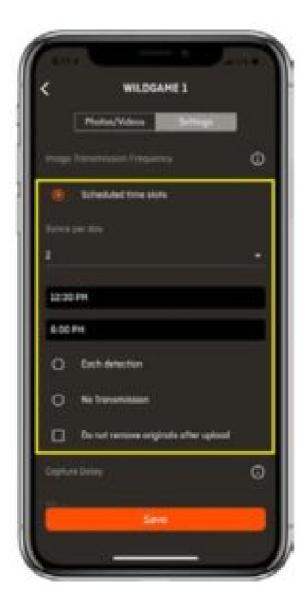
**Note:** Image transmission frequency greatly affects battery life. The more often the camera sends images, the quicker the battery will drain. For most efficient use, we recommend transmitting once or twice daily. Do not select the "each detection" function unless you are using a solar panel or some other battery source supplement.
