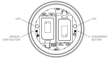
To enter Assignment Mode, press and hold the right button inside the WVL battery compartment for 2 seconds until the right (gear) LED lights up yellow.
