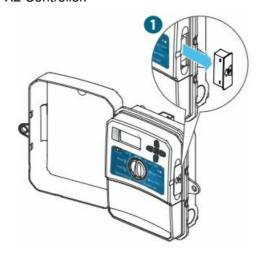
When installed, the WAND Module disables the X2 Controller's dial and button functions, the existing schedule, and settings.
