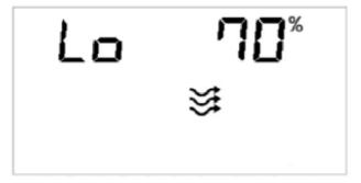
This also applies to each individual station and can be set from 20% to 90% using the + and – buttons. When this threshold is exceeded, the individual station will be shut down, an alarm will appear in the display, and the system will continue running the remaining stations in the program.
