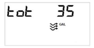
Total Overflow threshold is for catastrophic high-flow shutdown, and can be set from 1 to 1,000 GPM or I/min. This alarm applies to all stations and programs, shutting down all irrigation when the maximum threshold is exceeded.
