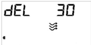
8. Press the right arrow button to access the **Delay** setting.
