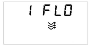
This will initiate a flow reading/calibration for each individual station and takes approximately 45 to 60 seconds per station. If there are individual stations that should be left out of the flow monitoring analysis, they can be set to OFF. You can also manually input or edit the nominal flows using the + and – buttons. To cancel the flow learning process, press the PRG button again to revert to the flow monitoring menus.
