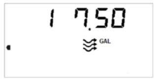
To access the nominal flows for each station in the system, press the right arrow button from the Delay menu. Cycle through all stations using the left and right arrow buttons to view or manually input all expected flow rates.
