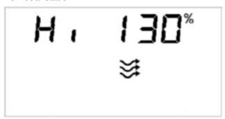
When this threshold is exceeded, the individual station will shut down, an alarm will appear in the display, and the system will continue running the remaining stations in the program.
