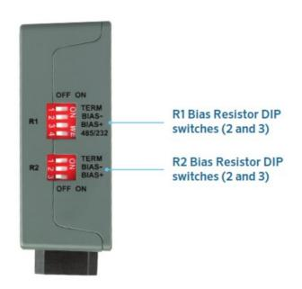
To enable Bias Resistors, move both the BIAS- and BIAS+ dip switches to the right in the orientation shown above. The bias resistors are used to keep the RS-485 bus to a known state, when there is no transmission on the line (bus is idling), to help prevent false bits of data from being detected. The bias resistors typically pull one line high and the other low – far away from the decision point of the logic.
