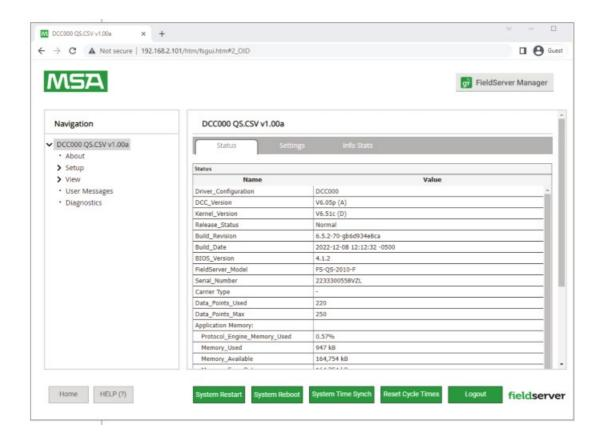
NOTE: The Field Server Manager tab allows users to connect to the Grid, Hunter Industries's device cloud solution for IIoT. The Field Server Manager enables secure remote connection to field devices through a Field Server and its local applications for configuration, management, and maintenance. For more information about the Field Server Manager, refer to the MSA Grid – Field Server Manager Start-up Guide.
