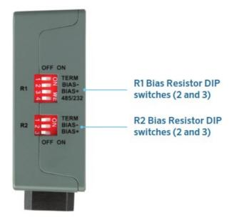
If the gateway is the last device on the serial trunk, then the End-Of-Line Termination Switch needs to be enabled. To enable the Termination Resistor, move the TERM dip switch to the right in the orientation shown above. Termination resistor is also used to reduce noise. It pulls the two lines of an idle bus together. However, the resistor would override the effect of any bias resistors if connected.
