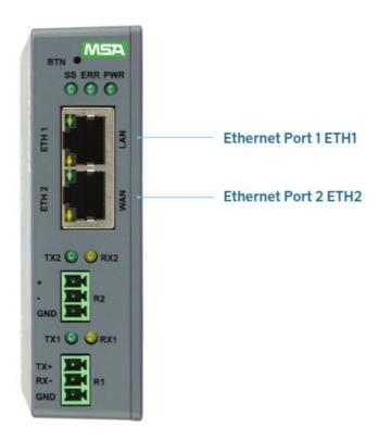
The Ethernet port is used both for BACnet/IP communications and for configuring the gateway via the Web App. To connect the gateway, either connect the PC to the router's Ethernet port or connect the router and PC to an Ethernet switch. Use Cat-5 cables for the connection.
