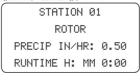
To simplify setup, several standard types of irrigation devices are included, along with typical precipitation rates. Select the type closest to the irrigation for the zone.
