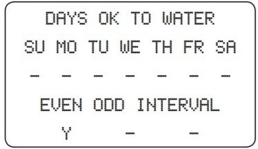
positions will change to a dash [-]. ET System will only permit water- ing on the selected Even or Odd dates in this position.
