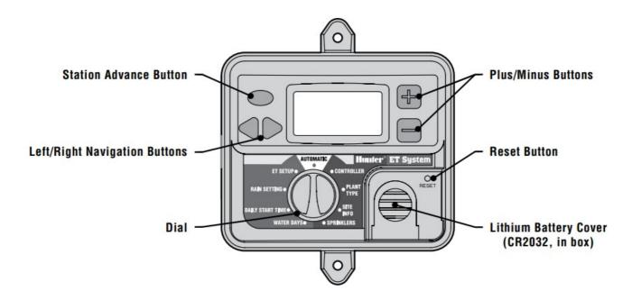
The ET Module has a backlit LCD display, a dial, and 5 buttons. There is also a recessed Reset button, and a removable lithium battery cover.
