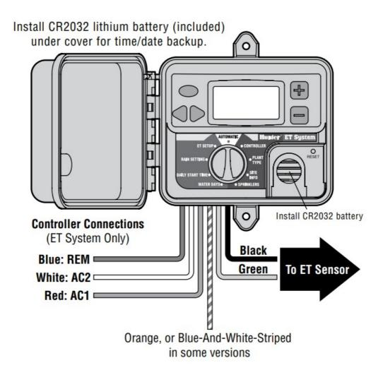
ET Module to the ET Sensor with appropriately sized butt splices or wire nuts. These two wires may be extended up to 100 ft./30m to reach the sensor.
