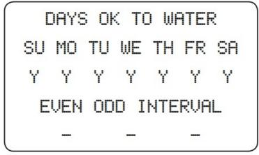
All days will initially be set to Y (Yes). The first day (Sunday) will be highlighted. To change the Y to N (No), use the +/- keys. Set any days on which you are not allowed to water, or don't wish to water, to . When the Y/N setting is
