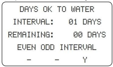
Interval, and the interval settings will replace the Day of Week display. You may set from 1 to 31 day intervals. Use the arrow keys to move to the Interval field, and press +/- to set the Interval.
