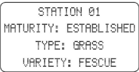
Set all information for one zone (or station), then advance to the next station with the Station button on the ET Module.
