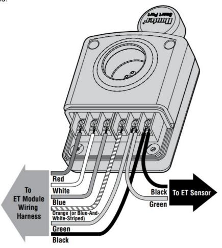
Twist the ends of the black wires from the ET Sensor and the ET Module together, and connect them together to the last terminal as marked.
