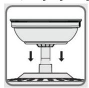
4. Choose the hanging system to the right that most closely resembles the one used by your fan and place the receiver as shown.
