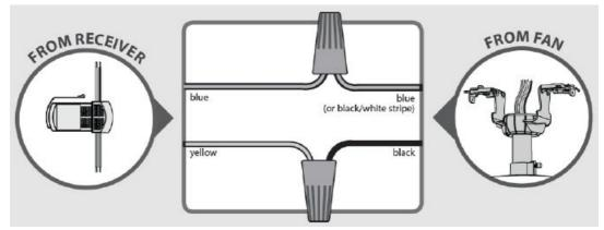
6. Connect wires from the receiver and fan to wires from the ceiling as shown. Using the wire connectors, connect the black wire (ungrounded) from the ceiling to the black wire from the receiver. Connect the white wire (grounded) from the ceiling to both the white wire from the receiver and the white wire from the fan. If you're uncertain about wire colors or connections, please contact a qualified electrician.
