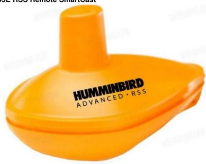
There are two versions of the RSS that are available: Channel A and Channel B. When using the A or B version of the RSS, make sure to select the appropriate channel for the RSS in the Channel menu on your control head. The A or B RSS option is intended to give you the flexibility to change to a different RSS and channel if another angler is using a SmartCast product in close proximity.
