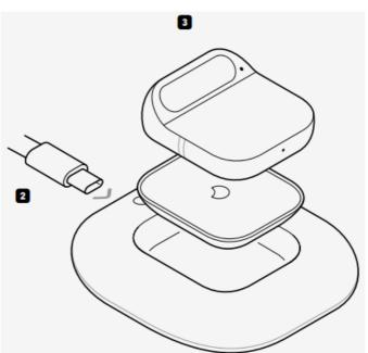
3. When it's time to charge the Battery Booster, place it on the Charge Pad. Make sure the Charge Pad is connected to the Humane-provided Adapter and Cable.
