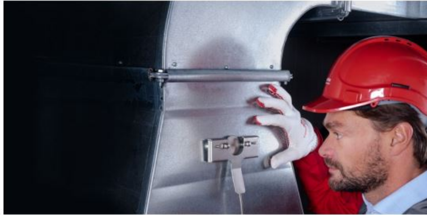
Figure 7 Mounting of IHF02 using an optional frame with magnets: note that optical properties of the sensor (black) do not match those of the metal object on which the sensor is mounted. This will lead to bad measurement data. (see also figure 3).
