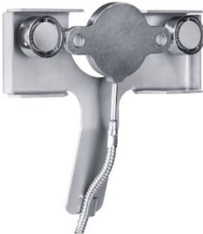
Figure 7 Mounting of IHF02 using an optional frame with magnets: note that optical properties of the sensor (black) do not match those of the metal object on which the sensor is mounted. This will lead to bad measurement data. (see also figure 3).
