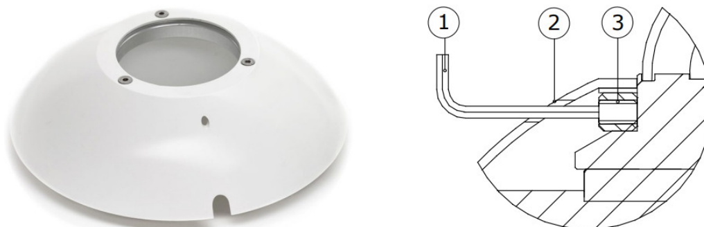
Figure 5.2.1 SCR01 sun screen and its installation and removal: turn the set screw using the hex key and lift off the sun screen to remove. (1) hex key, (2) sun screen, (3) set screw
