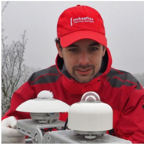
Figure 0.2 Heated to counter frost and dew deposition: clear difference between a non-heated pyranometer (back) and SR30 with RVH Liabilities covered: test certificates TM technology (front).
