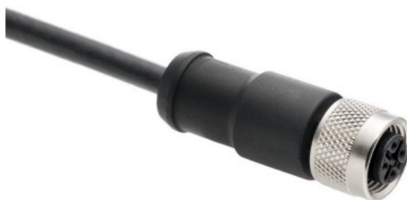
Figure 0.8 SR30 standard cable with M12-A female connector on sensor end. On the opposite end (not visible), the cable is terminated with removed sheath over 0.15 m; stranded copper conductors with plastic insulators, stripped ends with ferrules. Its length is 5 metres standard and it is available in 10 and 20 metres too.
