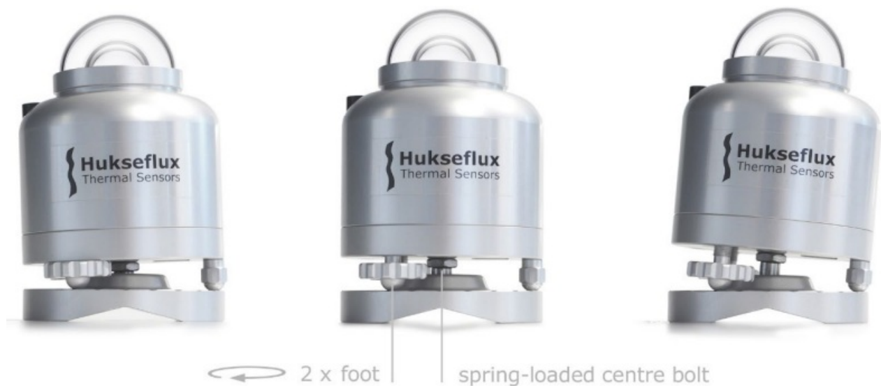
Figure 5.3.1.5 SR30 locked on its optional levelling mount: by fastening (on the left) or loosening (on the right) SR30's two adjustable feet, SR30 can be levelled, judging by the bubble level. SR30's static foot remains fixed. In all cases, ensure the legs of SR30 fit into one of the small ledges of the levelling mount. Locking is in place, when the nut is turned all the way against the bottom plate of SR30.
