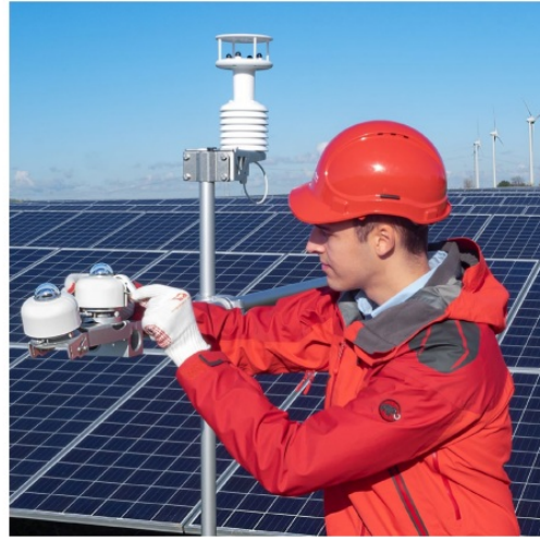
Figure 0.2 Heated to counter frost and dew deposition: clear difference between a non-heated pyranometer (back) and SR30 with RVH Liabilities covered: test certificates TM technology (front).
