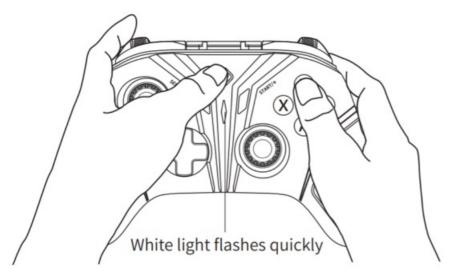
**Bluetooth connection:** Enter the pairing interface on the SWITCH host, and the host will automatically pair. After successful pairing, the host will automatically assign a channel, and the corresponding channel indicator will be on.
