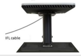
5. Ground the user terminal via the IFL cable using the provided ground block. For grounding requirements, see OneWeb HL1100W UT Installation Guide (1044008-0001).
