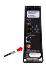
7. Connect the DC power cord to the IDU's DC IN connector and apply power by connecting the AC power cord to the surge protector, as shown.
