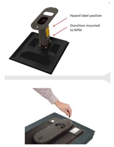
4. Thread one end of the IFL cable onto the antenna type F connector.
