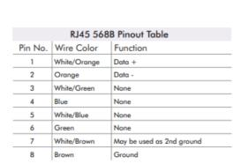
RJ45 568B Connection Pinout
