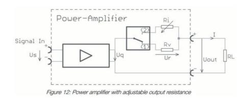
Amplifier output resistance: Rv  $\approx$  17 m $\Omega$  (different for each amplifier / see data sheet)
