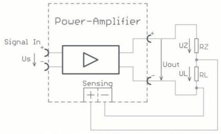
Figure 10: Exemplary test setup with sensing option used
