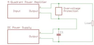
Figure 1: DC- and AC-Source (4-Quadrant Power Amplifier) in Series Operation
