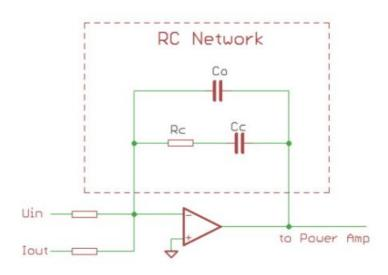
Figure 9: Simplified Current Controller
